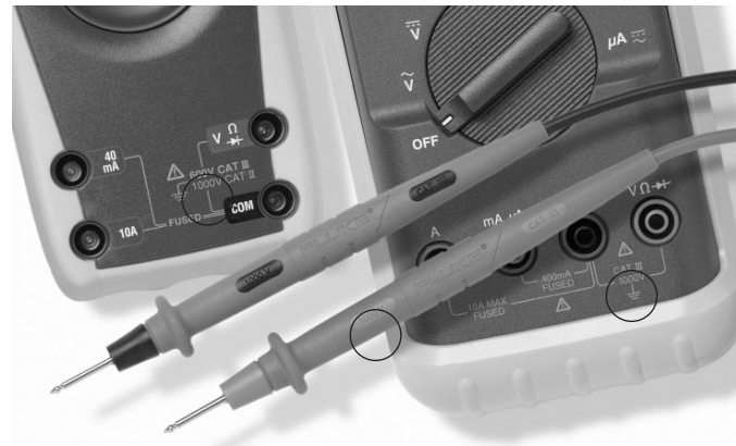
Look for category and voltage ratings of test leads and multimeters.
